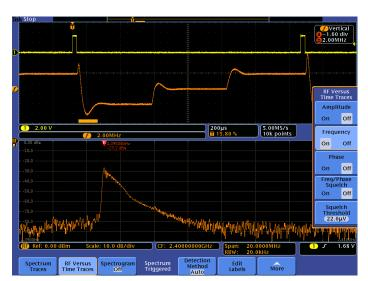
The orange waveform in the Time Domain view is the frequency vs. time trace derived from the RF input signal. Notice that Spectrum Time is positioned during a transition from the highest frequency to the lowest frequency, so the energy is spread across a number of frequencies. With the frequency vs. time trace, you can easily see the different frequency hops, simplifying characterization of how the device switches between frequencies.
