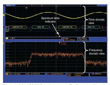
The upper half of the MDO4000 Series display shows the Time Domain view of the analog and digital channels, while the lower half shows the Frequency Domain view of the RF channel. The orange bar - Spectrum Time - shows the period of time used to calculate the RF spectrum.
