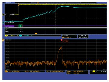
Figure 2 - Spectrum Time is moved about 60 µs to the right. At this point, the spectrum shows that the PLL is in the process of tuning to the correct frequency (2.400 GHz). It has made it up to 2.3168 GHz.
