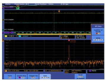
Capture - Triggering on a specific transmit data packet going across a SPI bus. A complete set of triggers, including triggers for specific serial packet content, ensures you quickly capture your event of interest.
