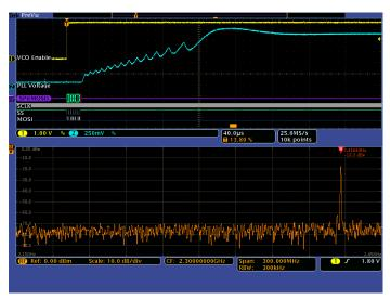
Figure 3 - Spectrum Time is moved another 120 µs to the right. At this point the spectrum shows that the PLL has actually overshot the correct frequency and gone all the way to 2.4164 GHz.
